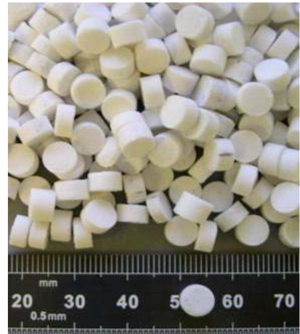
Pellets capturing CO 2 using amine polymer
